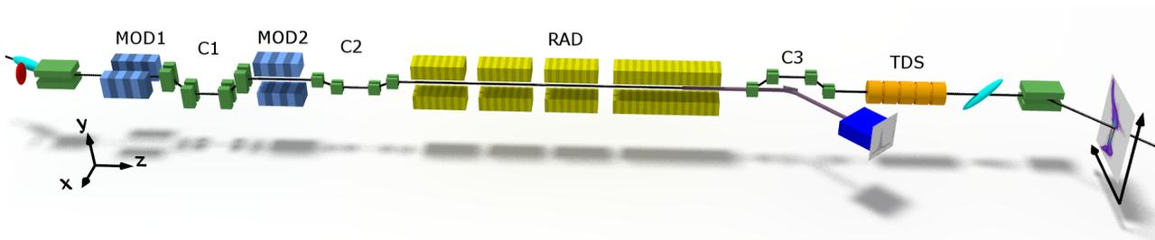
Figure 1: Layout of the sFLASH seeding experiment.
