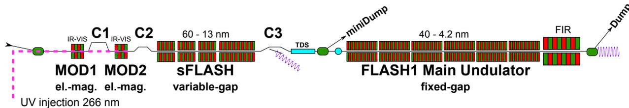
Figure 1: Layout of the FLASH1 beamline.
