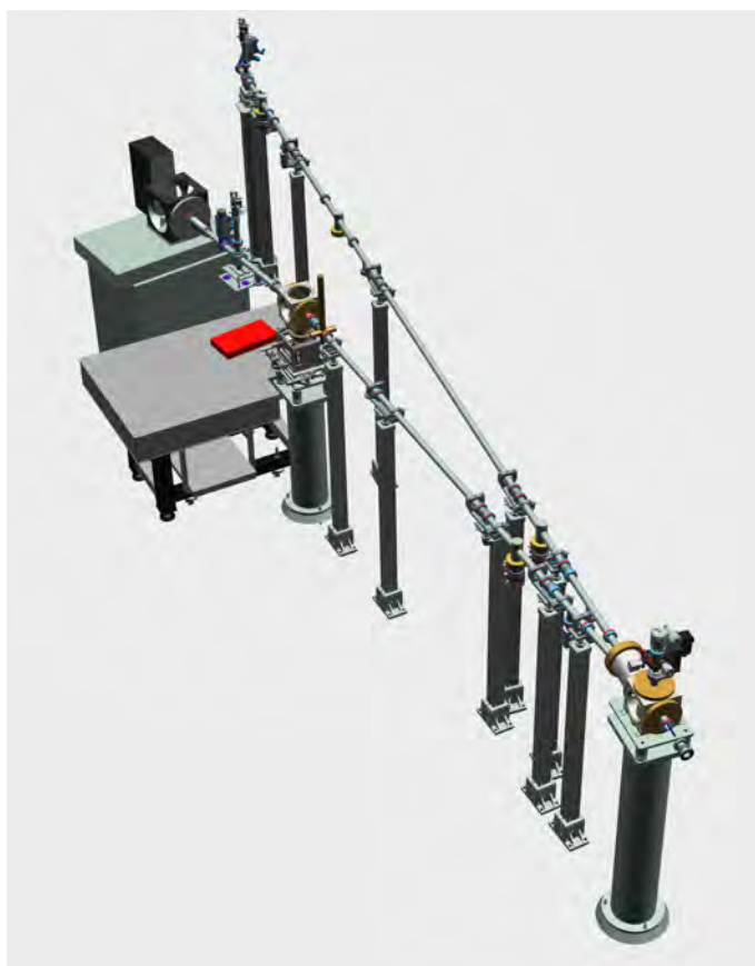
Figure 7.9: End of beamline FL21 with two branches: pulse length diagnostics (left) and open port for exploratory setups (right).
