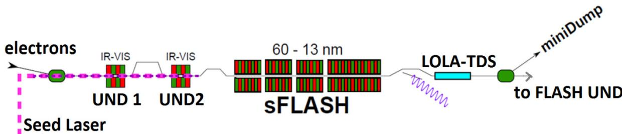
Figure 3: Arrangement of the FLASH1 seeding section.
